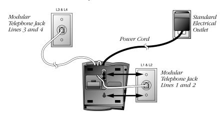
9 Plug the power adapter into a standard electrical outlet not controlled by a wall switch.
