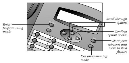
• Press PROGRAM to enter the programming mode. The screen displays:
