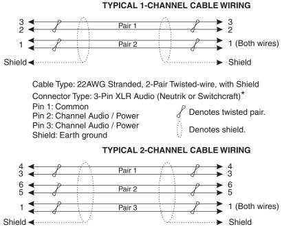
Cable Type: 22AWG Stranded, 3-Pair Twisted-wire, with Shield
