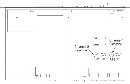
Figure 2 - Locations of Configuration Jumpers and Switches
