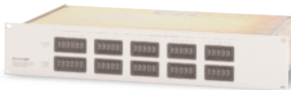
Source assignment panel. Assigns any one of 12 intercom channels and/or three program audio channels to 26 separate 2-channel user stations via convenient matrix thumb wheel switches. I/O provided via two 50 pin connectors. Normally used in conjunction with a BOP-220
