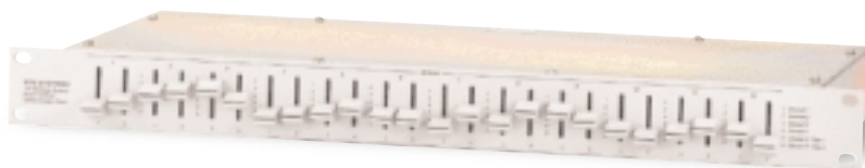
Source assignment panel. Transforms a basic two bus intercom system into a 6 bus system via convenient matrix slide switches. Provides six input channels and 24 output channels. I/O provided via two 1/4 inch, three 3 pin XLR female and twelve 3 pin XLR male connectors. Contains XLR jacks for RTS power supply.
