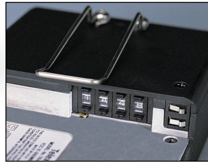
Code Switch: Allows operator to select up to 65,000 different cipher codes (BTR-600 set only).
