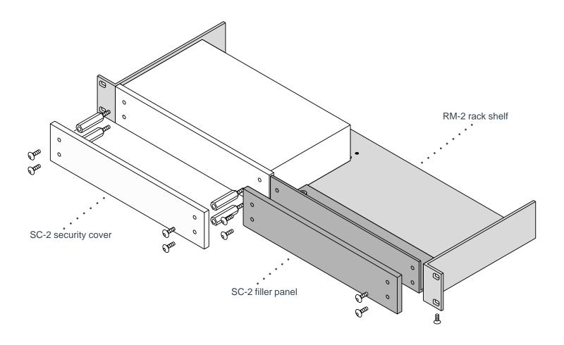
**RM-2** rack shelf is drilled from flush front or recessed mounting of two SX200 series products in a single rack space. Mounting screws included.
