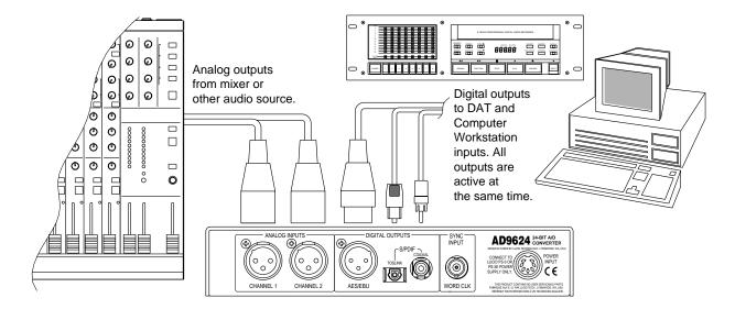
Figure 3-1. AD9624 Connections
