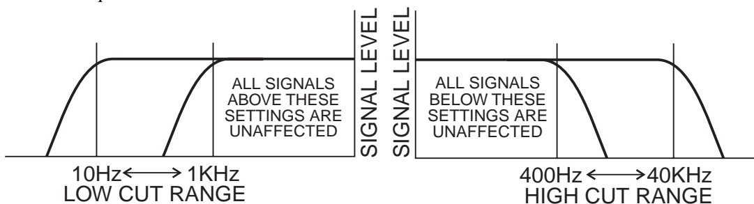
Frequency ranges of the Low CUT and HIGH CUT sidechain filter controls.
