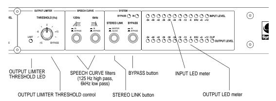
OUTPUT LIMITER THRESHOLD LED-Indicates peak limiting activity.
