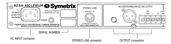
AC INPUT - This connector accepts nominal AC power sources of 115 volts or 230 volts [see Appendix A (Specifications) for voltage tolerance ranges]. See chapter 4 (Installation) for details on the detachable (IEC) power cable.
