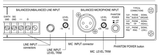
LINE INPUT - These connectors are electronically balanced, line level, bridging inputs. The 1/4" connector tip is high, ring is low, and sleeve is ground. The screw terminal input is wired in parallel to the 1/4" connector.
