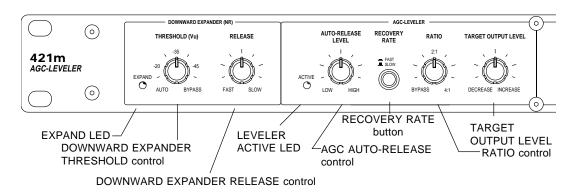
DOWNWARD EXPANDER THRESHOLD - Determines the level below which the downward expander operates, which reduces the gain at a 1:2 dB ratio.
