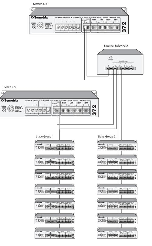
Connect a cable from EXT RELAY and Ground terminals of the master unit to the External Relay control and Ground terminals on the rear panel of the external relay.
