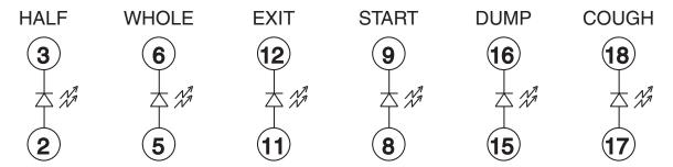
Note: The numbers within the circles refer to pins on the 6000's rear panel DB-25 connector which is labelled REMOTE INDICATOR & CONTROL INTERFACE.
