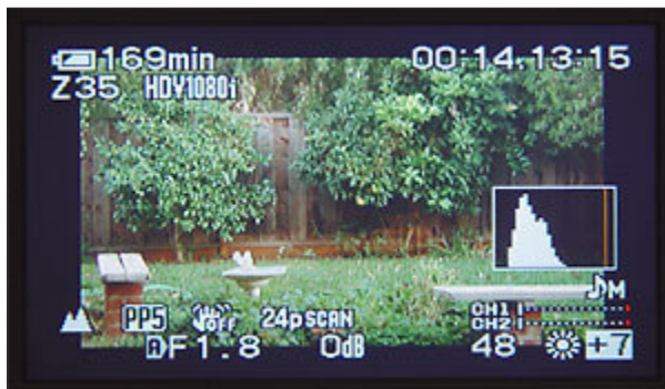
LCD in All-scan mode: all readouts shown (iris on auto, gain, shutter, and audio on manual), daylight with +7 warming, and histogram.
