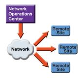
Operated from Sony's Network Operations Center (NOC) or your own internal NOC, Sony's DCDS allows for the centralized management and distribution of content packages (video, graphics, text) to remote sites for display on network players.
