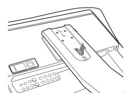
Remove four screws to remove the stand attachment bracket.
