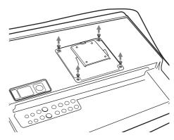
Attach the mounting bracket, then attach the unit to the rack with four screws.
