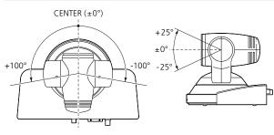
\* When the camera is panned more than 45 degrees with the camera tilted 25 degrees downward, the camera base might be in the field of view depending on the zoom setting.
