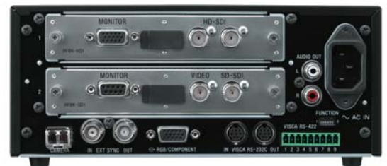
BRU-H700 rear panel with the optional HFBK-HD1/HFBK-SD1
