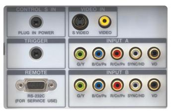
Versatile Inputs: rear connector panel gives you inputs for standard (composite) TV and video equipment, S-Video high-resolution components, RGB/Component video sources, RS-232C control systems, and Control S for home entertainment component integration.
