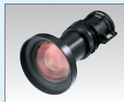
VPLL-FM20 Fixed short focus lens for 0 degrees optical axis angle installation (for rear projection), f 24.24 mm/F 3.0
