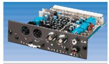
IFB-1000\*2 Composite/Y/C input (Loop-through BNC/ Loop-through Mini DIN 4-pin)
