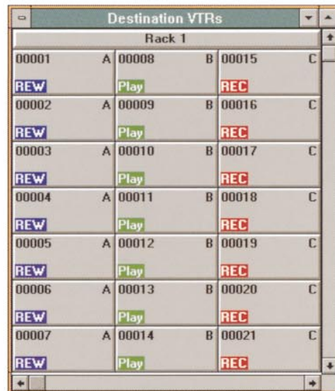
THE IDO SOFTWARE GIVES YOU A GRAPHIC REPRESENTATION OF YOUR DUPLICATORS, MUCH AS IF YOU WERE LOOKING AT THE RACKS THEMSELVES. EACH MACHINE IS IDENTIFIED BY RACK, ID NUMBER, AND GROUP.
