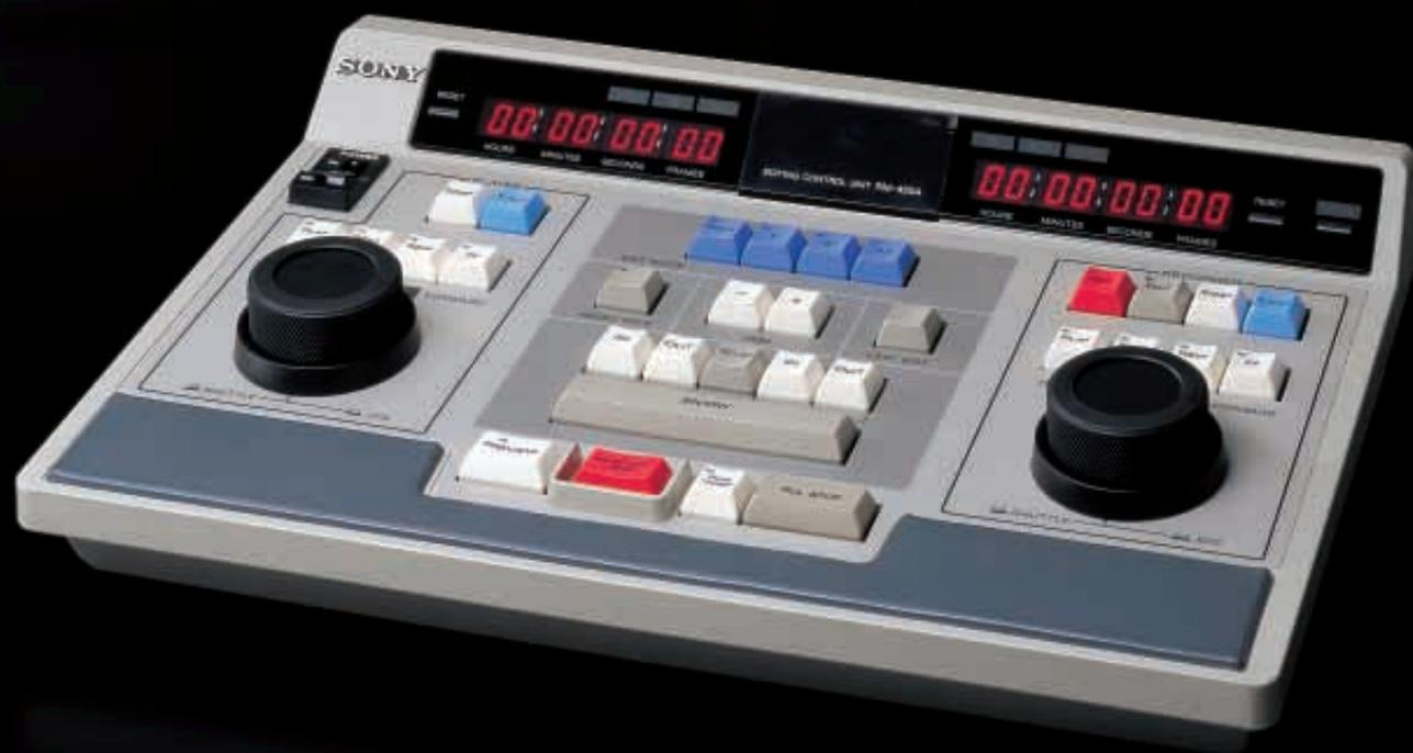
The Sony RM-450A Editing Control Unit is designed to make two-machine editing an easy and efficient operation.
