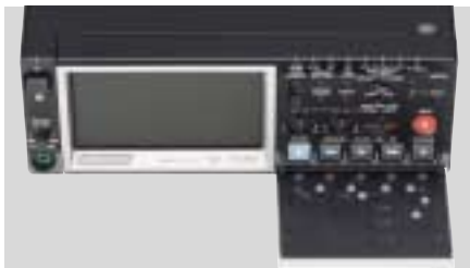
Control Panel Lid Open
