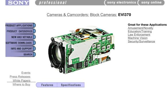
The EVI-370 CCD camera block incorporates a 1/3" (380k effective pixels) CCD. Up to 12 times optical zoom is available throughout the EVI-370 series.
