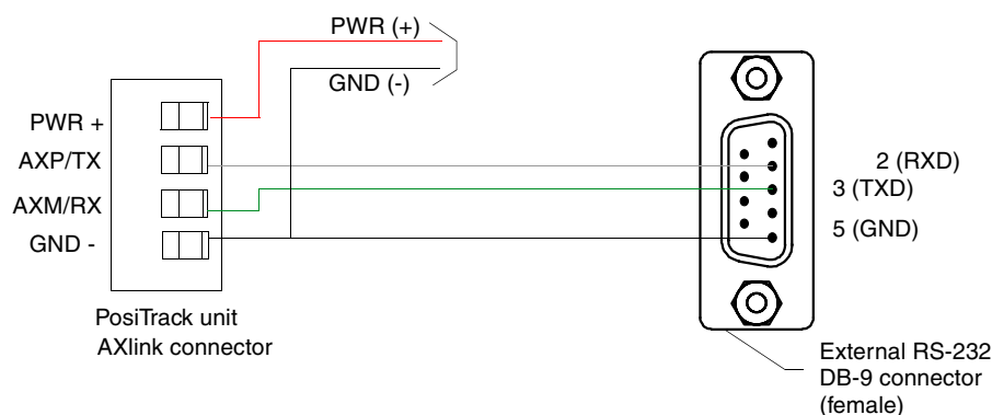
FIG. 23 External RS-232 control device or PC wiring diagram
