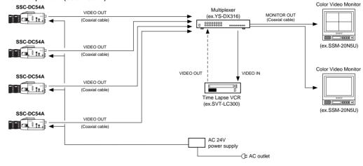
3. VBS lock operation (SSC-DC50A: DC 12V/SSC-DC54A: AC 24V)
