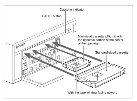
The cassette is automatically pulled into the operating position and the cassette indicator lights up.
