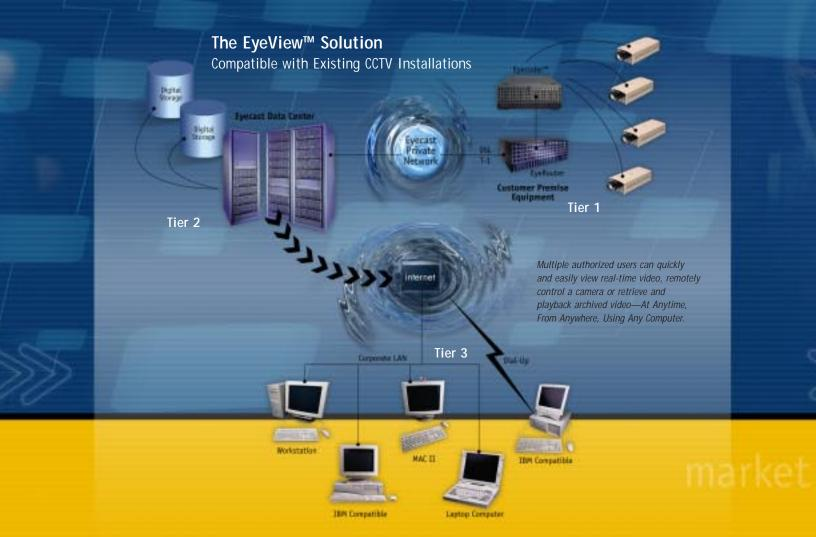
EYECAST provides end-to-end service to customer locations nationwide through our unique three-tiered architecture, which includes:
