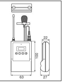
$63 \times 100 \times 27 \text{ mm} (2 \frac{1}{2} \times 4 \times 1 \frac{1}{8} \text{ inches}) (w/h/d)$  (excluding the antennas)
