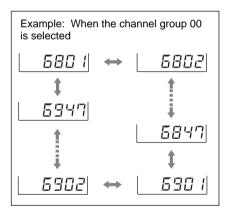
7 When the desired channel number appears, leave the tuner for about 10 seconds until the selected channel number stops flashing and the selection is stored in memory.
