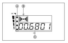
(A) **RF** (radio frequency) indications The number of dots indicates the RF input level.
