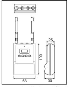
$63 \times 100 \times 30 \text{ mm} (2^{1}/_{2} \times 4)$  $\times 1^{3/16}$  inches) (w/h/d) (excluding the antennas) Approx. 180 g (6 oz) including batteries
