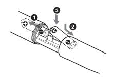
**3** Turn the grip in the direction opposite to the arrow in step 1 to close the battery compartment.
