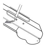
Attaching the supplied accessory to the handheld microphone (UTX-H1)
