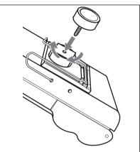
After attaching the belt clip and the shoe mount adapter, insert the microphone stand adapter into the screw hole at the top of the shoe mount adapter, and then rotate the microphone stand adapter until it is securely attached.
