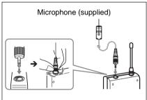
For a secure connection, be sure to turn and lock the connector cover.
