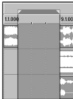
Result of Time Selection Cut without Ripple Edit Mode
