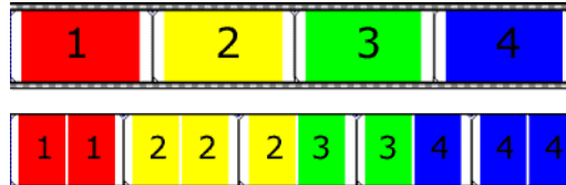
24 fps film (top) and resulting NTSC video with 2-3 pulldown fields (bottom)
