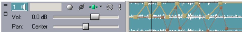
Figure 2.11 Automation envelopes applied to Track 1.
