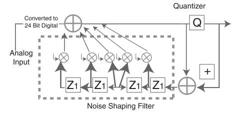
The Audible Improvement (which exceeds 10db) is in Noise Level! (for frequency ranges lower than 3 kHz)
