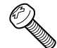
Screw (+B6 x L20) (2)/ Vis (+B6 x L20) (2)/ Tornillo (+B6 x L20) (2)
