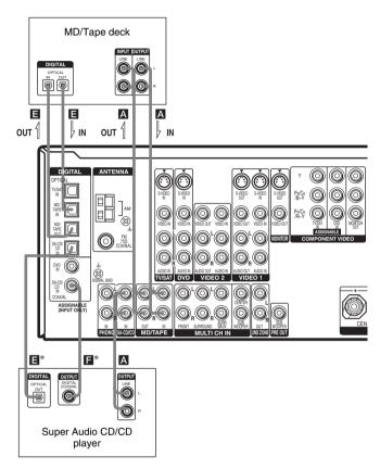
\* Connect to either the SA-CD/CD COAXIAL IN or the SA-CD/CD OPTICAL IN jack. We recommend making connections to the SA-CD/CD COAXIAL IN jack.
