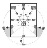
When placing two surround back speakers (The angle **G** should be the same)
