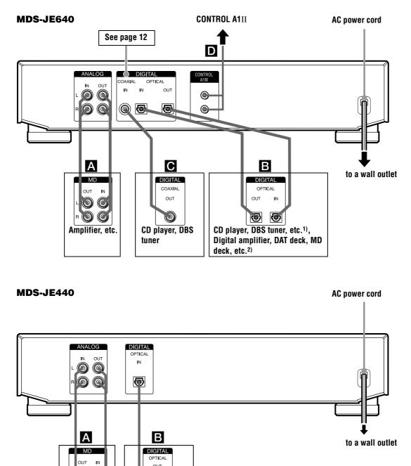
1) Digital equipment with a DIGITAL OUT connector only
