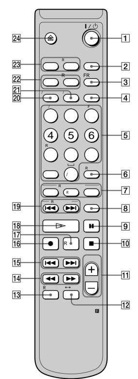
1 I/() (power) switch (13) (23) Press to turn on the deck. When you turn on the deck, the STANDBY indicator on the deck turns off. When you press the switch again, the deck turns off and the indicator lights up.
