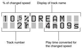
The time display at the display window is also displayed during conversion for the changed speed.
