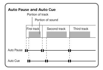
You can select the level (threshold level) of a sound in the Auto Cue position
