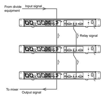
By the connection above, the input and output signals are ralayed, but for reasons of the system, the input signal is cut off for about 2 seconds when recording is relay. If you want to perform overlap recording without a blank, connect the input signal as shown below.
