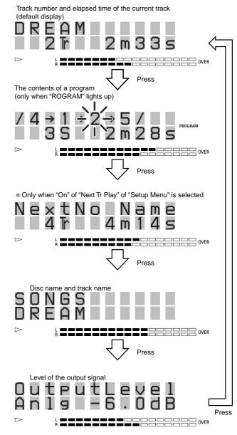
\* Not displayed if PLAY MODE is PROGRAM or SHUFFLE when "On" of "Next Tr Play" (Next Track Play) is selected. You can check the remaining time Press TIME. Each press of the button changes the display as follows:
