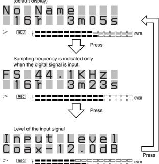
You can check the remaining recordable time on the MD Press TIME when the track number and recorded time are displayed. Each press of the button changes the display as follows:
