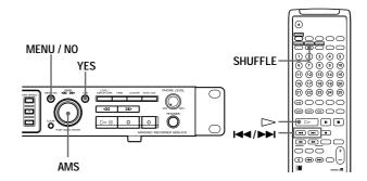
1 Press SHUFFLE while the recorder is stopped. "SHUFFLE" lights up at the display window.
