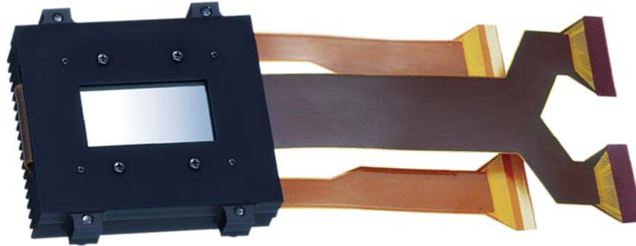
More than 8 megapixels on an inch and a half of silicon, this is the professional version of Sony's SXR™ device.
