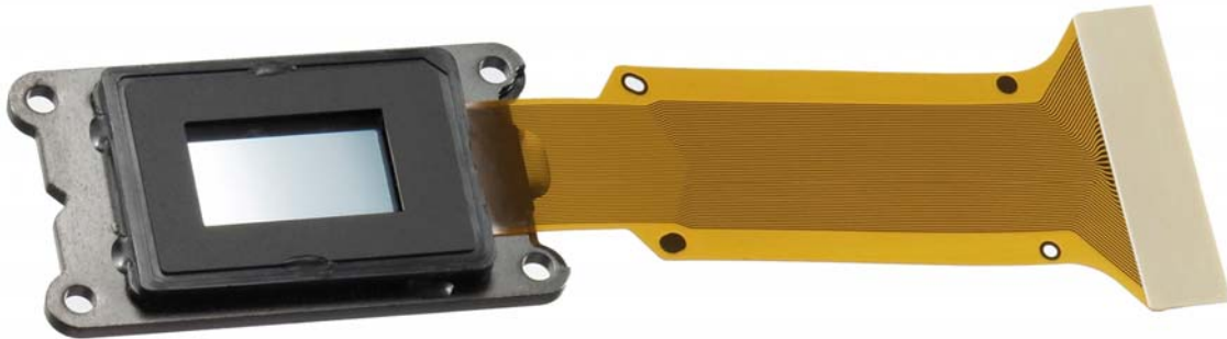
Sony's third-generation SXRDTM device, key to the KDS-R60XBR1 and KDS-R50XBR1.
