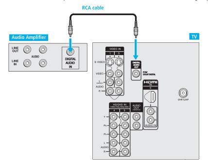
Because all equipment does not output digital audio, you should also connect the TV's analog audio output jacks to the amplifier's analog audio input jacks, as described on page 16.
