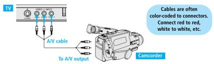
If you have a mono camcorder, connect its audio output jack to the TV's L MONO audio jack.
