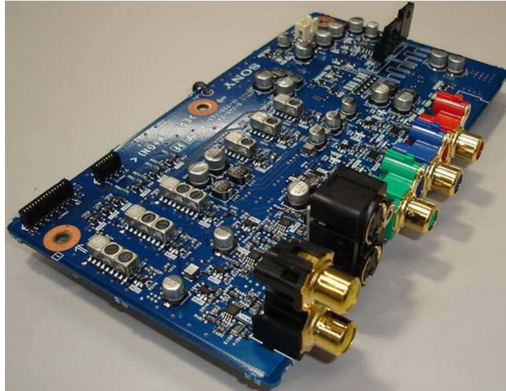
To maintain the purity of the signal, Sony places the analog video circuitry on a separate board, driven by its own power supply.
