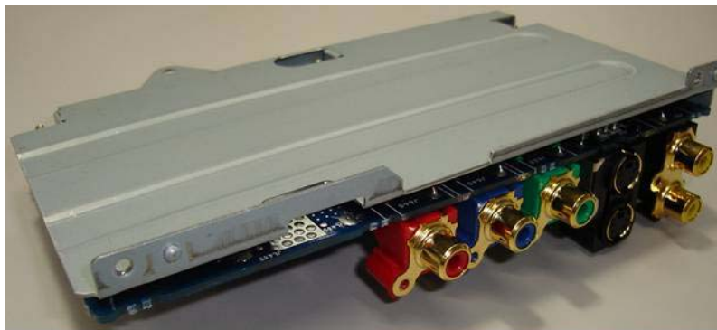
To minimize signal interference, the DVP-NS9100ES has a shield plate fitted to the underside of the analog video circuit board.
