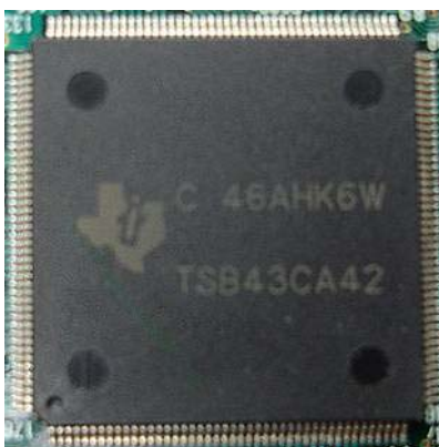
The i.LINK output circuit incorporates this Large Scale Integrated circuit from Texas Instruments.
