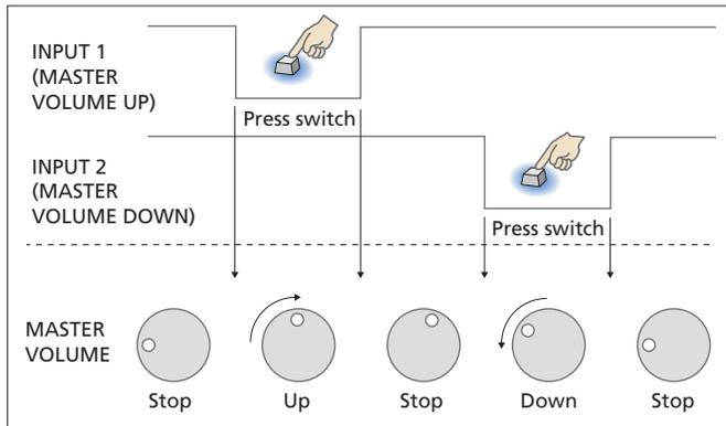
Fig. 11 Switch and MASTER VOLUME Status
