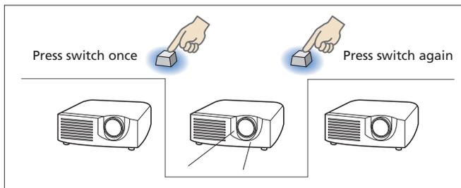
Fig. 5 Projector POWER ON/STANDBY Status
