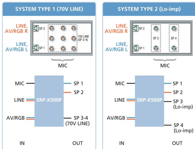
When using high-impedance ceiling speakers
