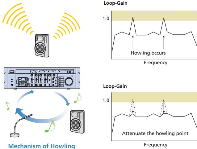
Mechanism of Howling
