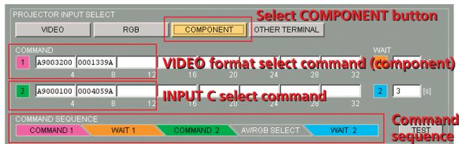
In this way, the SRP-X500P can send two commands at a time when selecting the input signal on the projector. However, it is also necessary to add wait time between one command and the next.
