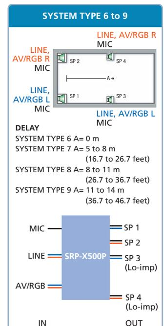
When using front speakers and satellite speakers
