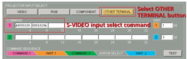
To select OTHER TERMINAL, it is necessary to select any one of the AV/RGB INPUT A to E buttons. Set any input to OTHER TERMINAL in SIGNAL DEFINE, as shown in Fig. 19 on page 22. (In Fig. 19, INPUT C is selected to OTHER TERMINAL.)
