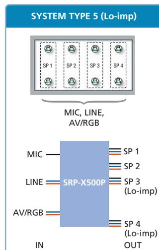
When using low-impedance ceiling speakers
