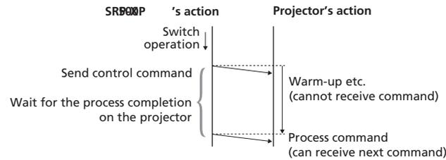
Fig. 20 Control Sequences to Control a Projector
