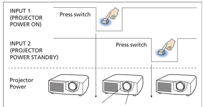
Fig. 7 Switch and Projector Power ON/STANDBY Status
