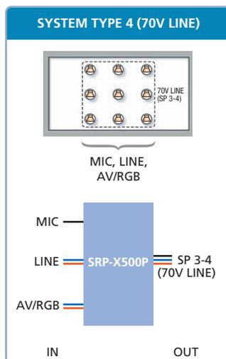
When using high-impedance ceiling speakers
