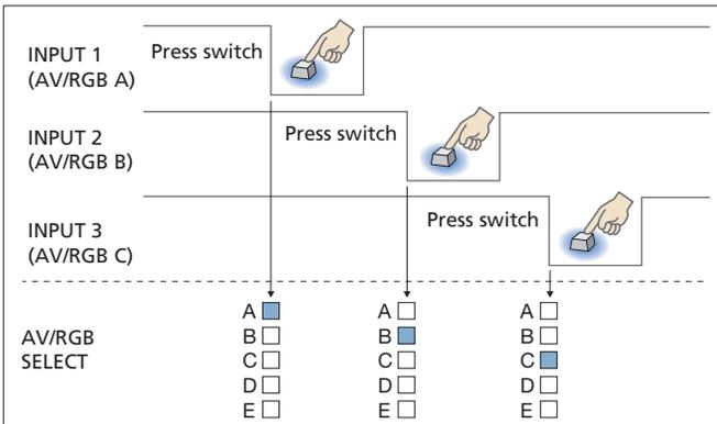
Fig. 9 Switch and AV/RGB SELECT Status
