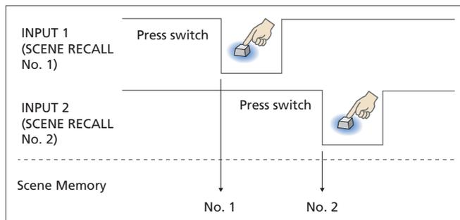
Fig. 13 Switch and SCENE RECALL Status
