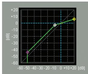
6. Adjust the GATE THRESHOLD level so that the gate does not open with the ambient noise level present during a presentation.
