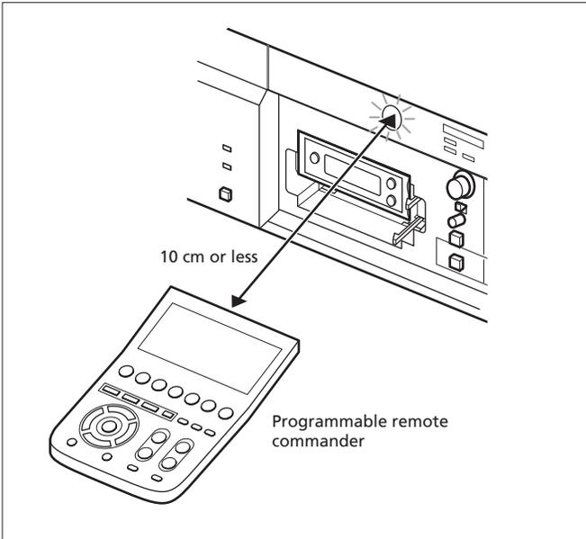
4. Press the IR OUTPUT MODE button. The button and the remote emitter/sensor flash, and commands are output from the remote emitter/sensor.
