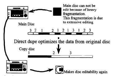
5) The information from the main(master) units is based on the TOC information on the disc, however duplication is possible in program mode, ram toc edit mode, and single play mode.
