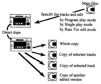
In any case, TOC information corresponded of the playback mode, will also be recorded on the DISC in the sub units.
