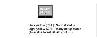
Normally, this button is dark yellow (READY/SAFE setup is off). In this case, the buttons, controls and switches directly control the audio processing.
