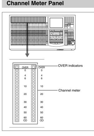
The channel meters indicate the input signal level of the channel strips.
