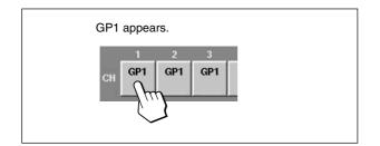
To remove the channel from the group, touch this button(s) on which the group number is displayed. The group number disappears and that channel is removed from the group.
