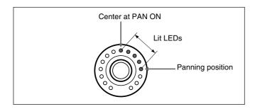
When PAN is OFF: Only the LED corresponding to the panning position is lit. When the panning position corresponds to the center LED, all LEDs are off. When functions other than panning (AUX, TRIM and MTR) are selected, the LED corresponding to the volume level is lit.
