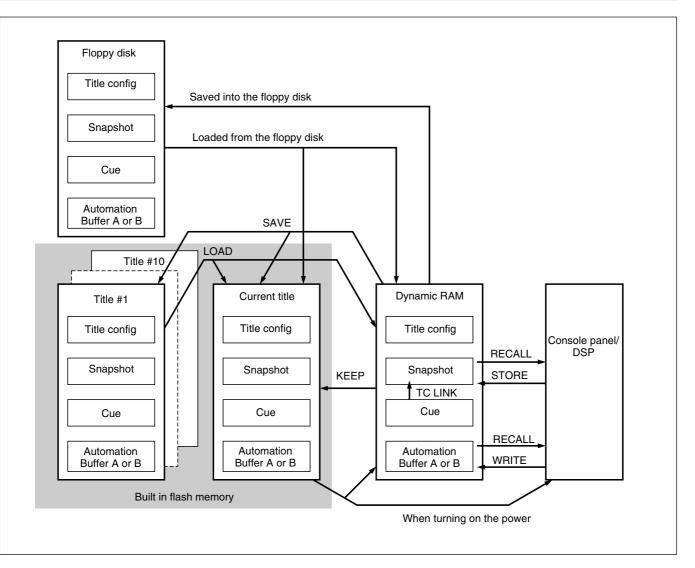
The above figure shows the memory structure of the unit. Automation data, snapshot data and cue data created on the unit are stored, updated and deleted on the dynamic RAM. Thus, when restarting the unit or turning off the power of the unit, this data is lost.
