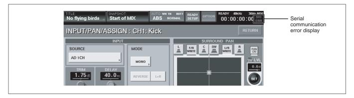
When the console is used as a cascade master unit or a cascade sub unit, SIO ERR is displayed in red on the error display area if any error occurs in communications using the PC port. Also, the
