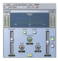
The DeNoise module is complex with 19 different controls, but most of it is fairly intuitive. In a dark-blue window in the upper third of the module, there's a display of the audio spectrum from 0 to 20 kHz and level from 0 to -144 dBFS. The Noise Fingerprint is shown as a hyphenated line that approximates the contour of the spectrum of the noise. The current spectrum of the noisy audio appears as a jagged line.
