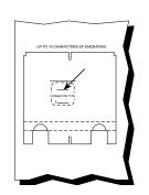
Indicate the desired text in the space provided above CONNECTOR TYPE. Up to 10 characters maximum per connector location is allowable\*\*.
