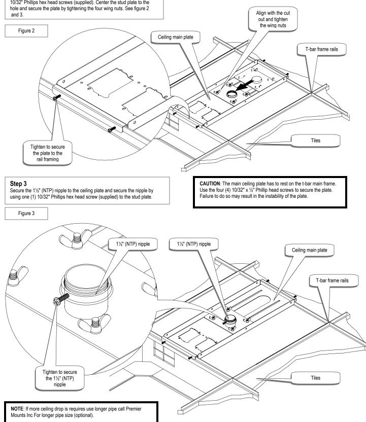
**CAUTION**: The 10/32" x  $\frac{1}{2}$ " Phillip hex head screw must be used to stabilize the  $\frac{1}{2}$ " (NTP) nipple or optional pipe.
