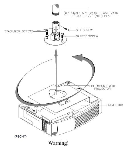
The wall/ceiling should be capable of supporting a weight of at least five (5) times the projector(s) or monitor(s)weight. If it cannot, the ceiling must be reinforced. Proper installation procedure by qualified personnel as outlined in the installation instructions must be adhered to. Failure to do so could result in serious personal injury.
