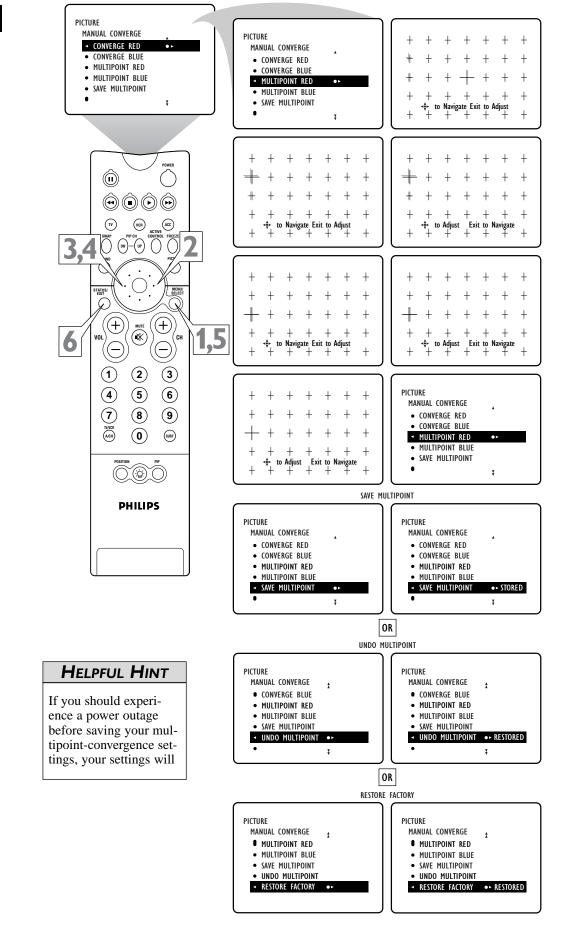
**Press the MENU/SELECT button**. The menu appears. Press the CURSOR RING RIGHT to enter the PICTURE menu. Then press the CURSOR RING DOWN until MAN-UAL CONVERGE is highlighted.
