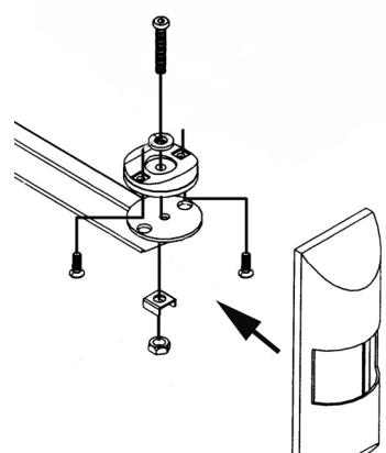
**3b)** Insert 5/16" platform screw (9) down through center of platform swivel bracket. Place platform swivel bracket assembly onto top plate at end of support arm, with main bolt passing through center hole.
