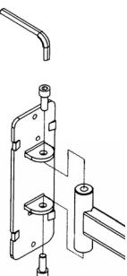
Insert support arm into wall bracket. Thread 3/8" pivot bolts into support arm, and secure with large hex wrench.
