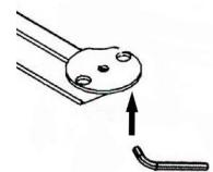
With tilt angle set, turn front edge of platform at right angles to support arm. Insert small hex wrench through holes in bottom of platform support as shown, and tighten tilt screws securely.
