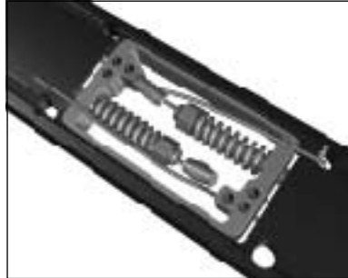
Cable Tensioning Assembly—showing assembled compression springs and cables.
